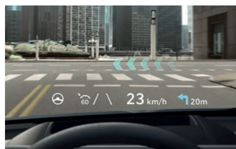
Augment-Reality Head-up Display
